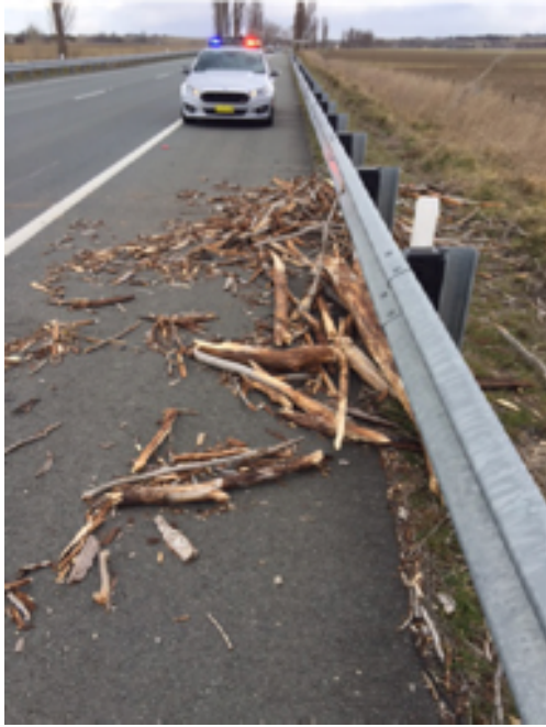
Figure 12a and 12b show the result of one of these trees falling on the carriageway. This is an unacceptable situation for road user safety, and also requires bringing maintenance crews and emergency service officers close to the carriageway each time a tree falls over and must be cleared. Over time the avenue had diminished and there was no plan to reinstate it in its current form.
